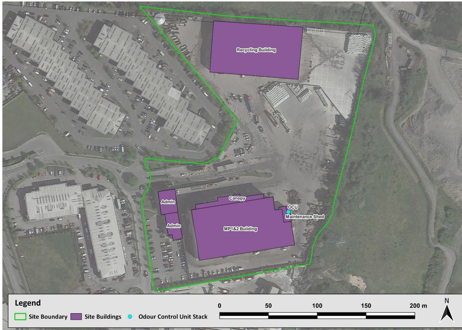
Figure 2 Material Recovery Facility site plan – identifying the layout of buildings at the site and the location of the proposed OCU.
